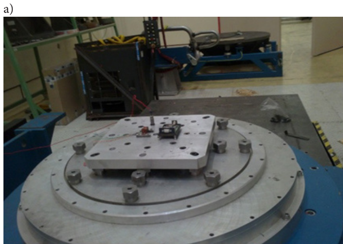
Figure 7. Mounting of the equipment on a vibration test jig a) set up for the transverse random test and b) for the longitudinal and vibration tests.
