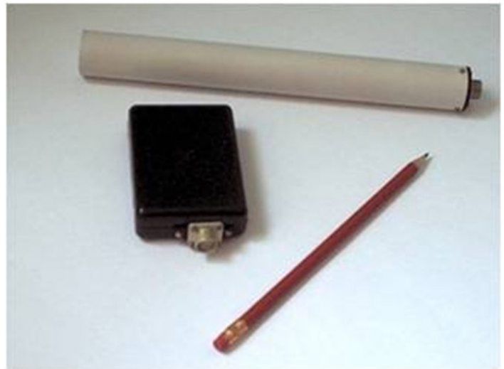
Figure 1. Pictures showing: a) the dimensions of MF_1D (adapted from the user's manual) and b) the LEMI-011 fluxgate magnetometers. LEMI-011B is the box (black) version and LEMI-011T is the tube (white) version.
