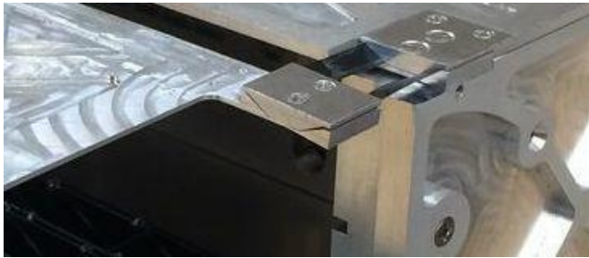
Figure 13. 30° Solid-State hinge configuration integrated into the ANDESITE 6U CubeSat.
