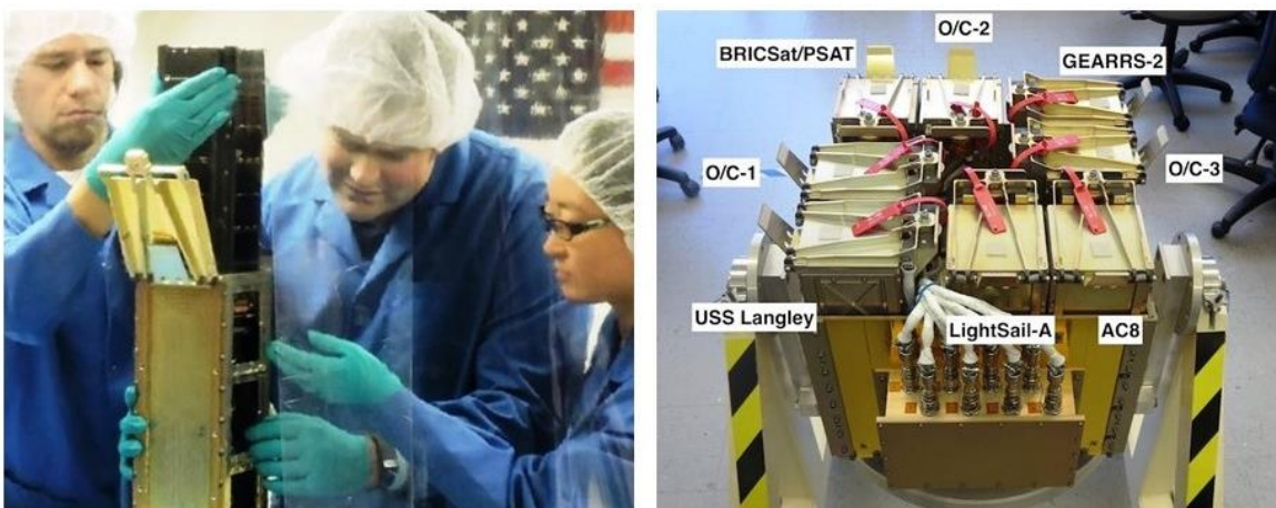
Figure 15. LightSail 1 integration into the P-POD (l) and ULTRASat fully loaded with P-PODs (r).
