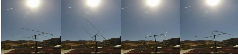
Figure 12. Cal Poly Ground Station Antennas tracking LightSail 1.
