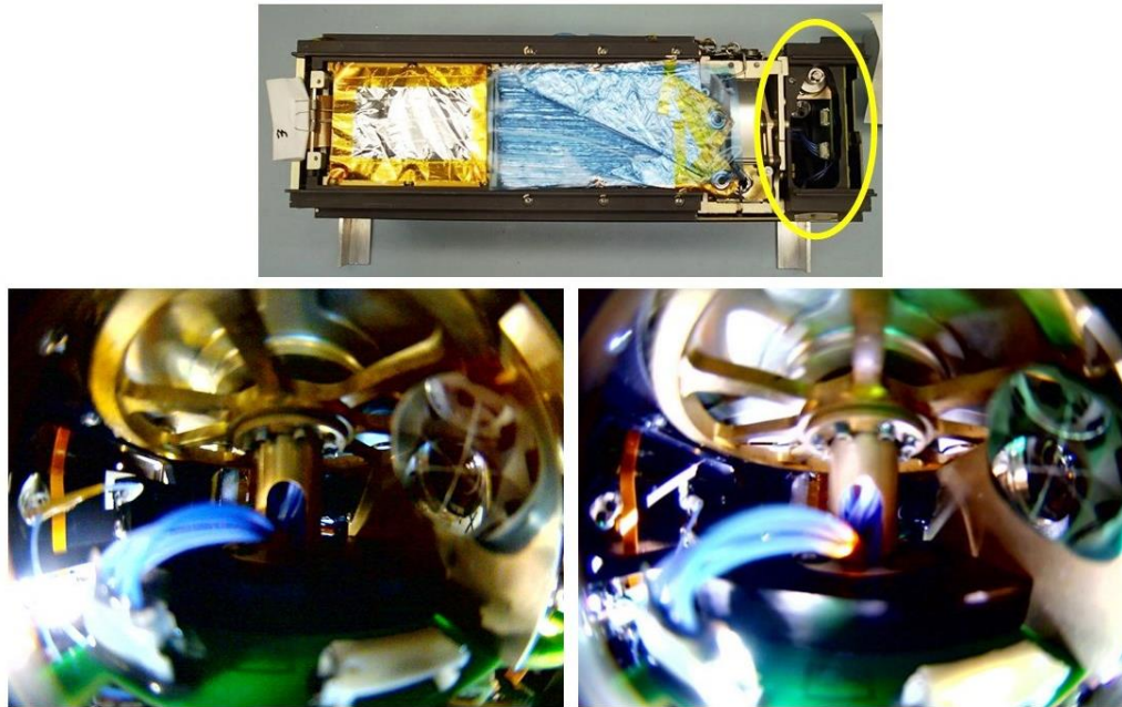
Figure 16. Results of test image in orbit (r) compared to one from lab-based system-level test (l).
