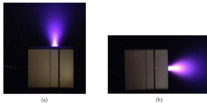
Figure 10. Plasma plume of the breech-fed PPT (a) and the side-fed PPT (b).
