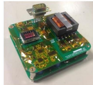
Figure 6. Power processing unit of the proposed dPPT.
